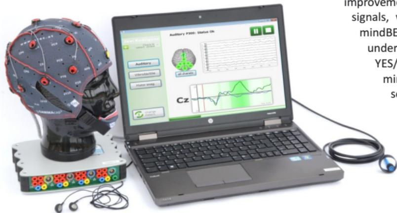
The mindBEAGLE® system consists of a portable medical grade biosignal amplifier, an EEG cap with active electrodes, a standard laptop computer with the mindBEAGLE® software, in-ear phones for auditory stimulation and vibro-tactile stimulators to be attached to the patient's body.
